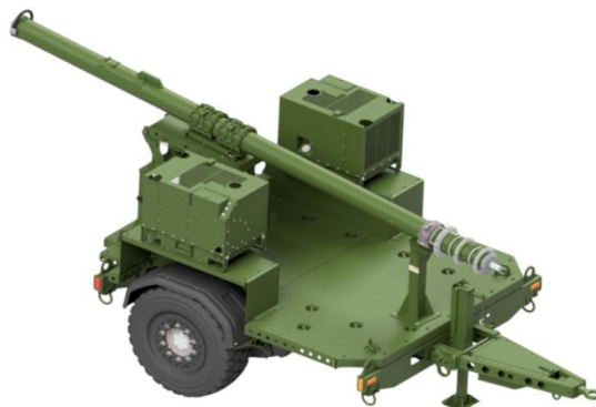
Typical 30m/34m Mast Installation on Contact's JLTV – Trailer Pallet System with twin LiquidPiston 10kW gensets
